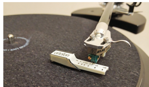
Photo of stylus force gauge to set tracking force
