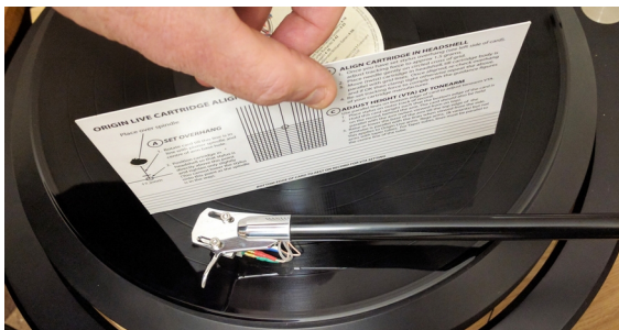
Above photo shows incorrect orientation of alignment card
